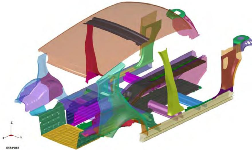
Figure 3-6 Components with Material Changes from T-5 Final to T5-D336
