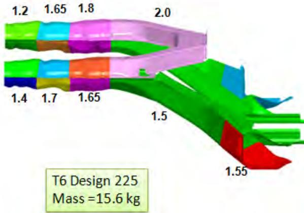
Figure 4-5: FSV T6 Final Front End Design and Material Gauges (TRIP 800)
