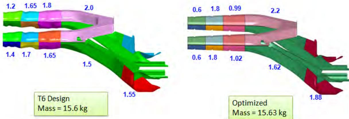
Figure 4-14: T6 Final Design (left) vs. Near-Term Optimized Design #73
