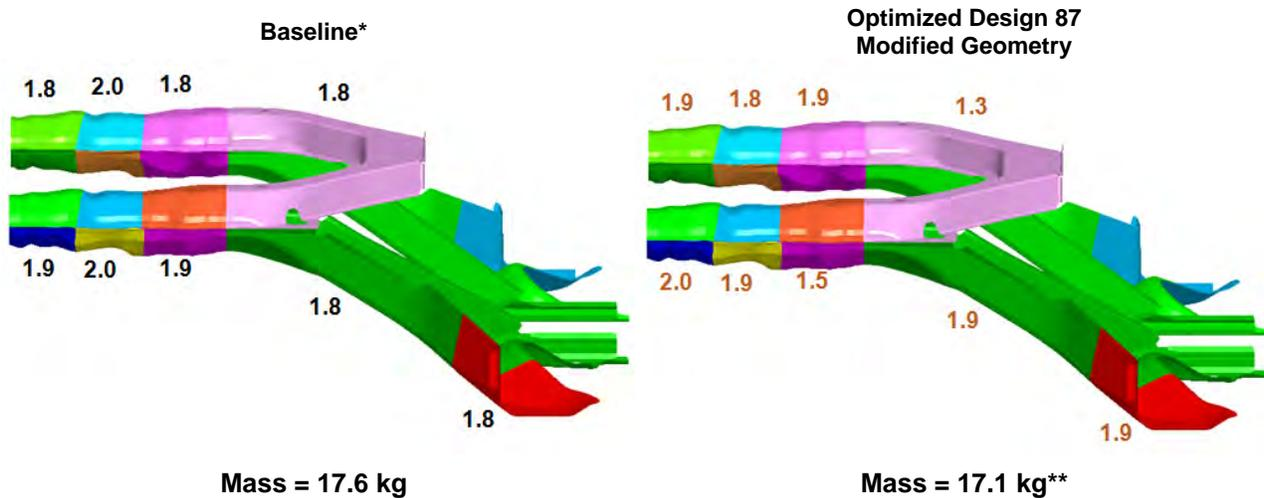
Figure 2-22: Modified Material Gauges, Design 87 Compared to Baseline
