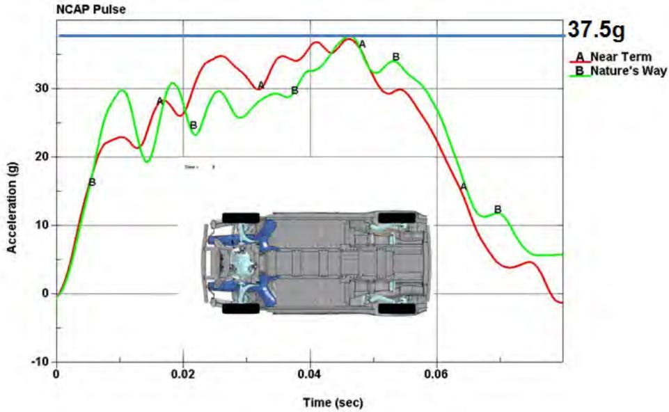
Figure 4-11: NCAP Pulse Results A) Near-Term Optimized Design vs. B) FSV T6 Final Design
