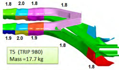
Figure 3-4: FSV T5 front rail subsystems
