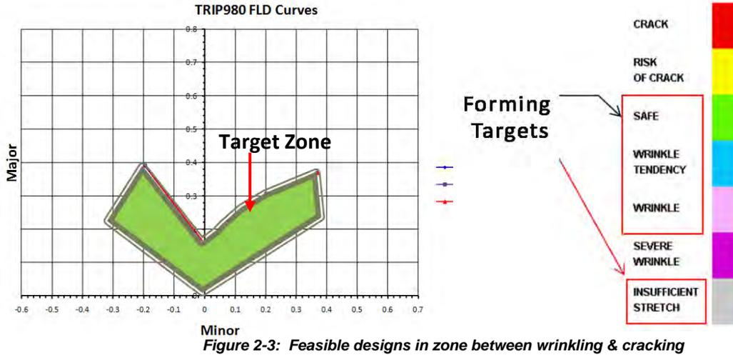
Figure 2-3: Feasible designs in zone between wrinkling & cracking
