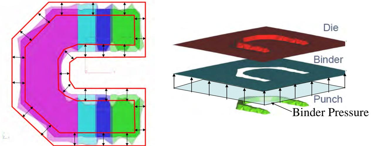
Figure 2-10: Blank geometry modification boundaries (left). Blank, Bead and Binder Pressure (Optimum Binder Force = 660 N/mm) are analyzed simultaneously (right)
