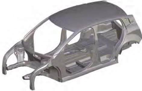
Figure 1-1: FSV BEV Body Structure
