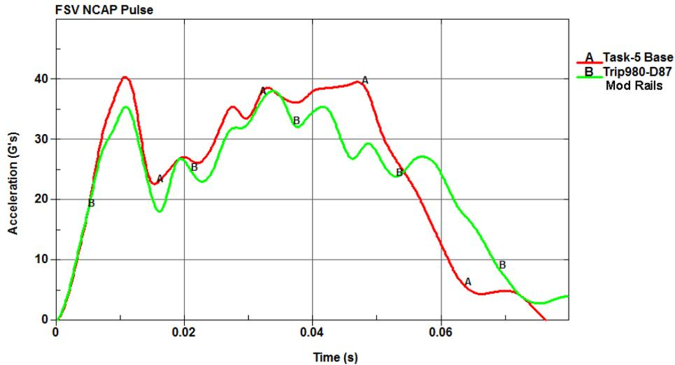
Figure 2-24: Results of Modified, Gauge Optimized Front Rails (green 'B' line) for US NCAP
