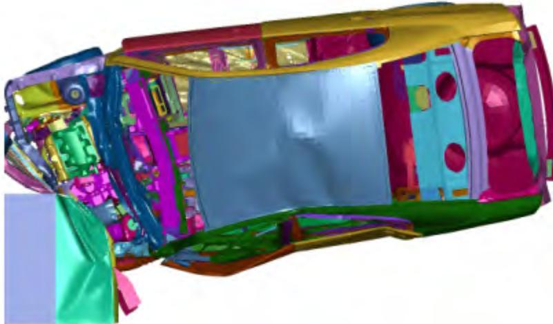
**Figure 12.25:** IIHS front 40% offset crash procedure
