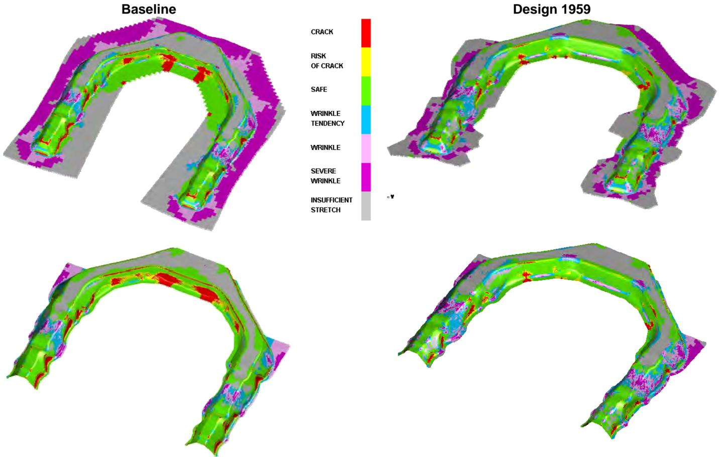
Figure 2-14: Design 1959 Upper Rail – 3B Forming Process Results
