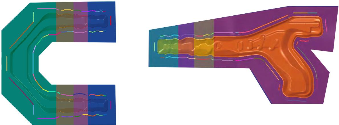
Figure 2-9: Line bead configuration for Upper Rail (left) and Lower Rail
