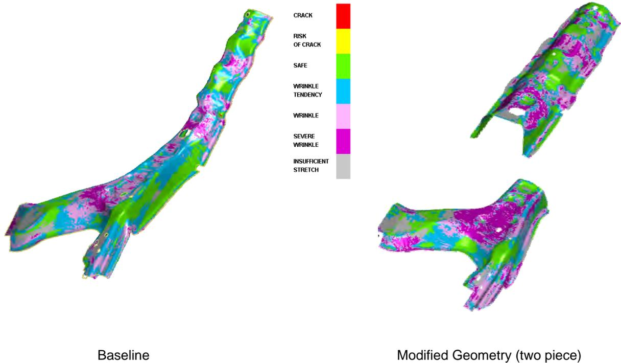
**Figure 2-26: TRIP 450/800 Baseline and Modified Geometry (two-piece) Lower Rail Forming Results**
