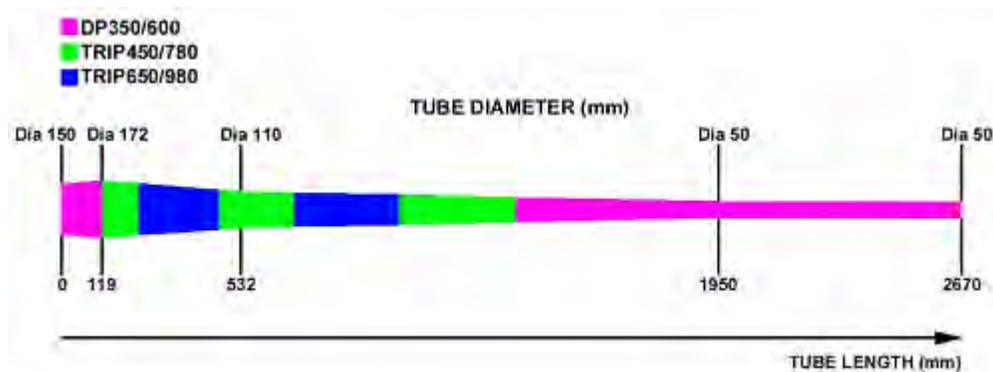
**Figure 12.32:** Final design hydroformed tube concept - geometry & material
