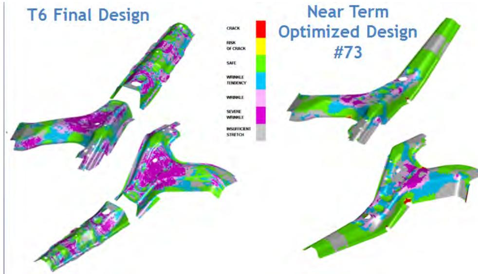
Figure 4-13: T6 Final Design vs. Near-Term Optimized Design #73 Formability
