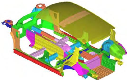
Figure 3-2: FSV parts that were updated according to T5 Design 336 Grades
