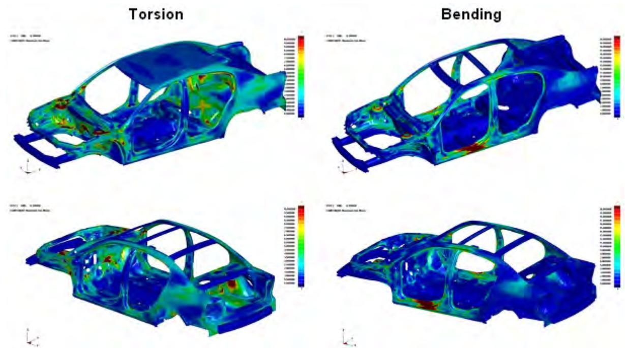
Figure 12.9: Static stiffness
