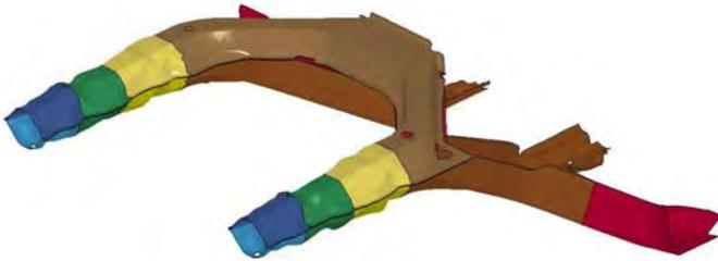
Figure 4-1: FSV Final Optimized Rail Design (T6)
