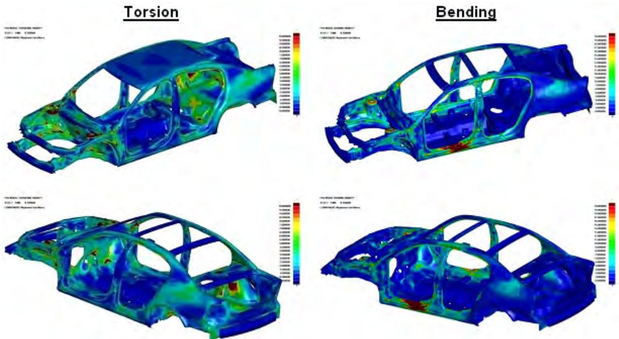
Figure 12.27: Static stiffness
