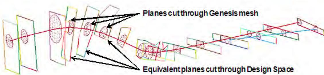
**Figure 12.14:** *Cross-sections through the Topology Optimization's load path mesh & design space*
