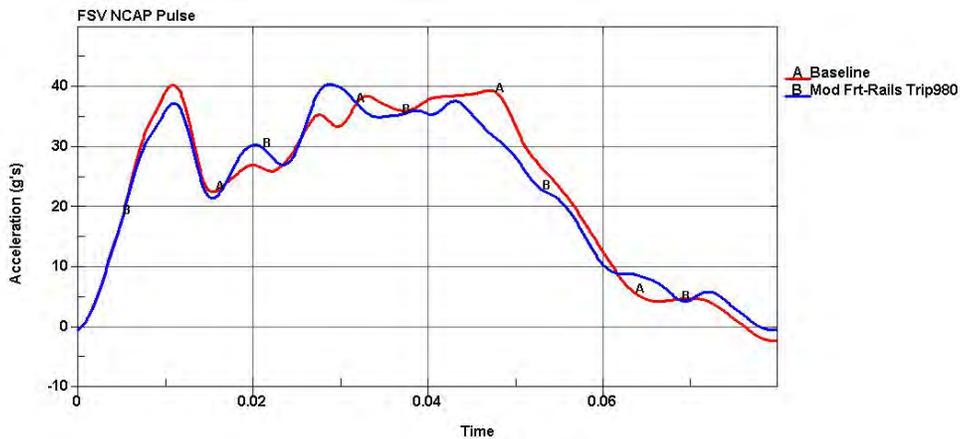
Figure 2-20: Modified Geometry US NCAP Performance Compared to Baseline
