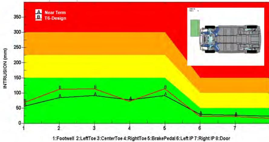
Figure 4-12: Near-Term Optimized Design (A) vs. FSV T6 Final Design (B)
