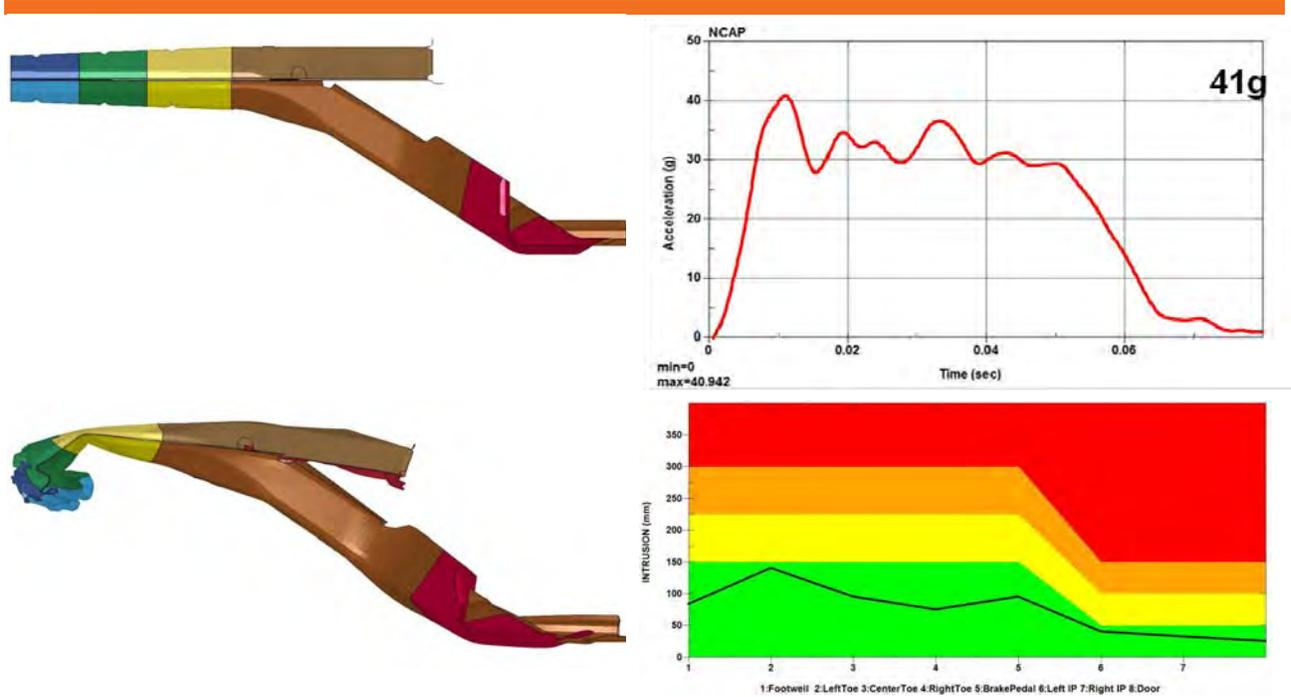
Figure 4:7: Crushed Rail (Bottom) and US NCAP (top right) and IISI ODB (bottom right) Results
