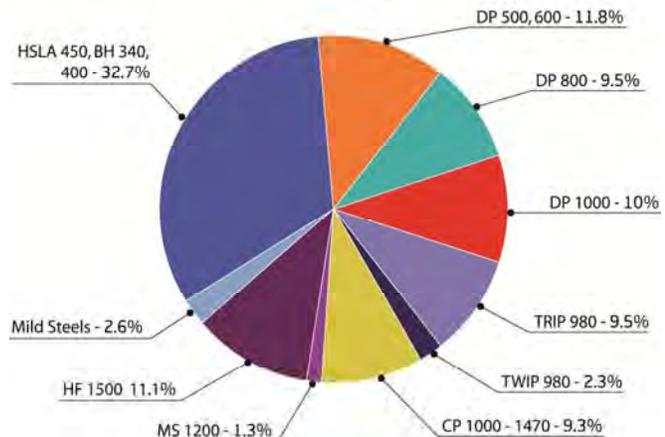
Figure 1-2: FSV BEV Body Structure and Steel Material Content
