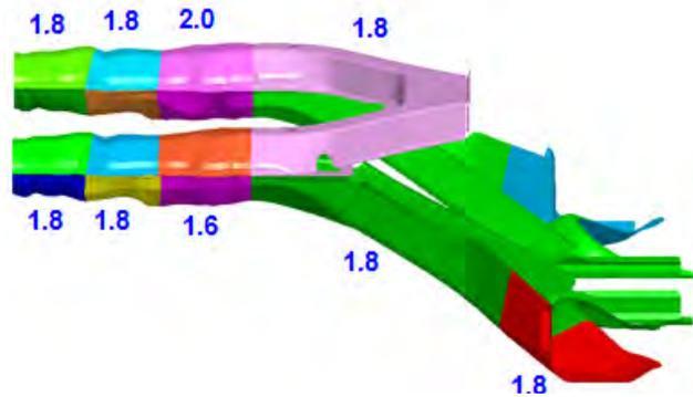
Design 66 Modified Geometry (two-piece Lower Rail) Gauges
