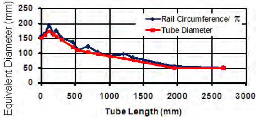
**Figure 12.30:** Final design hydroformed tube concept - equivalent diameters
