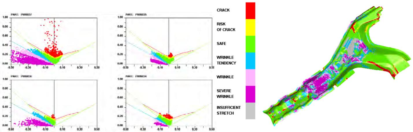
Figure 2-5: Baseline FSV T5 Design Lower Rail Forming Results
