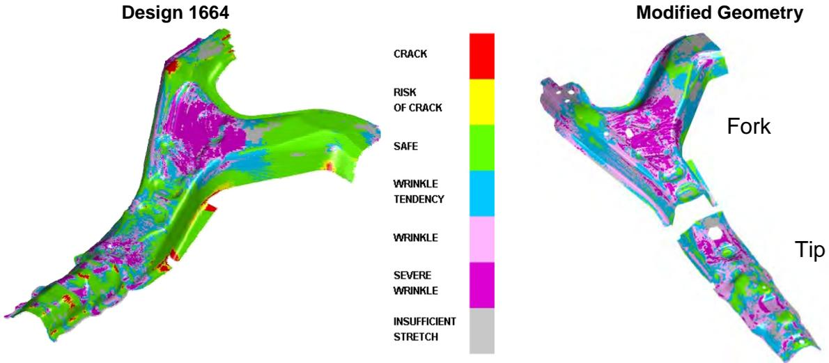
Figure 2-19: Lower Rail – 3B Forming Results on Modified Geometry
