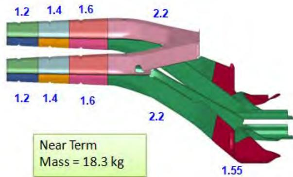
Figure 4-6: Near-Term Gauges (TRIP 800)
