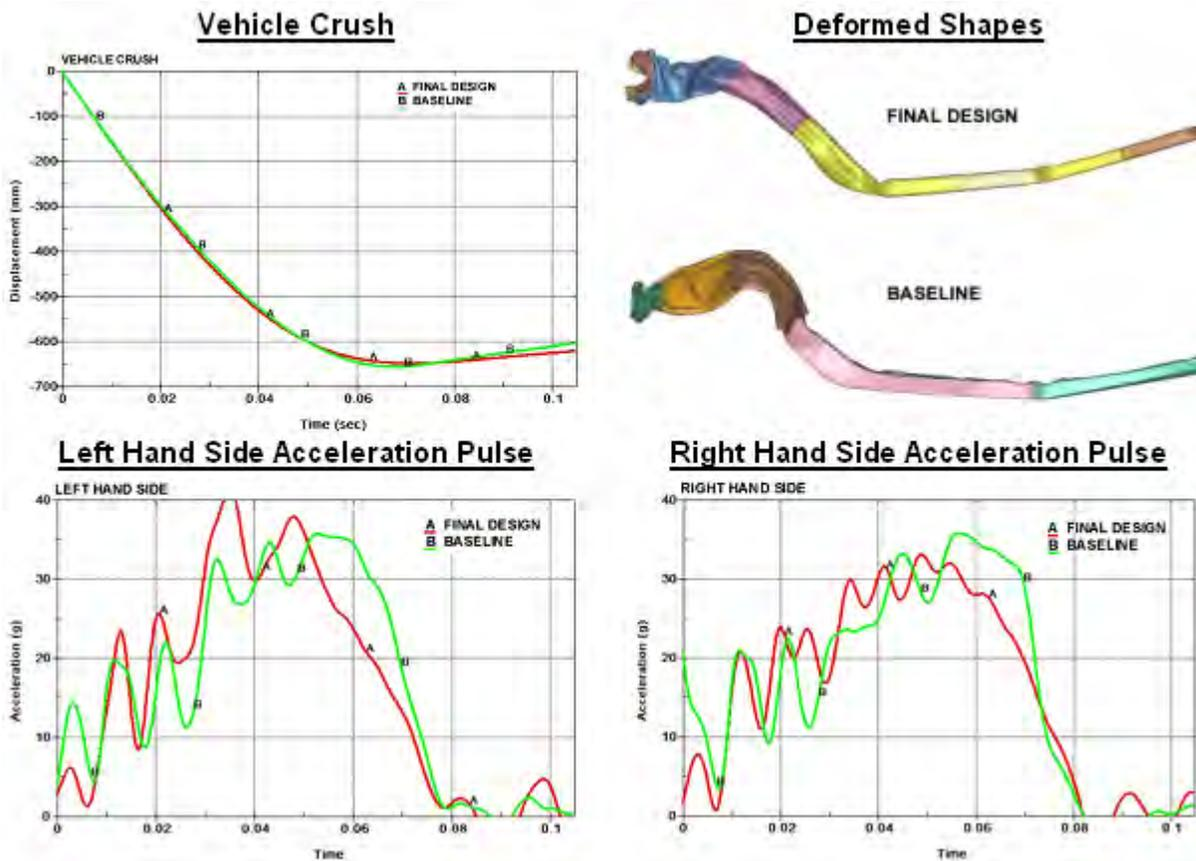
Figure 12.23: NCAP - final design & original rail - deformed plots & Acceleration
