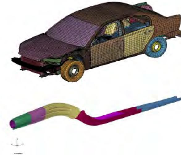
**Figure 12.5:** Model as received (front rails shown for clarity)
