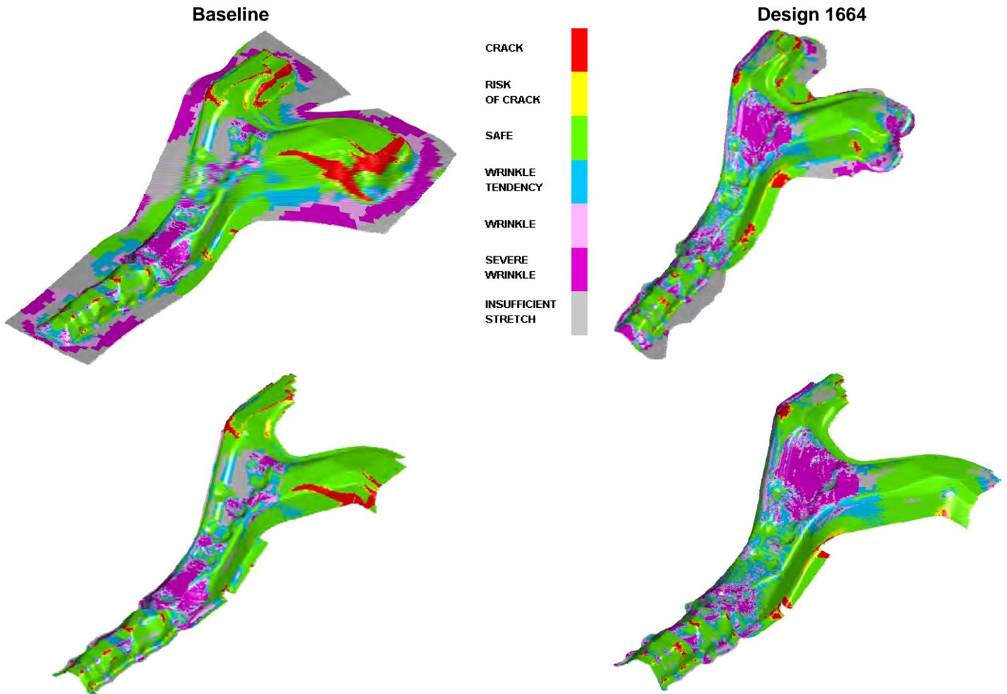
Figure2-15: Design 1664 Lower Rail Forming – 3B Forming Process Results
