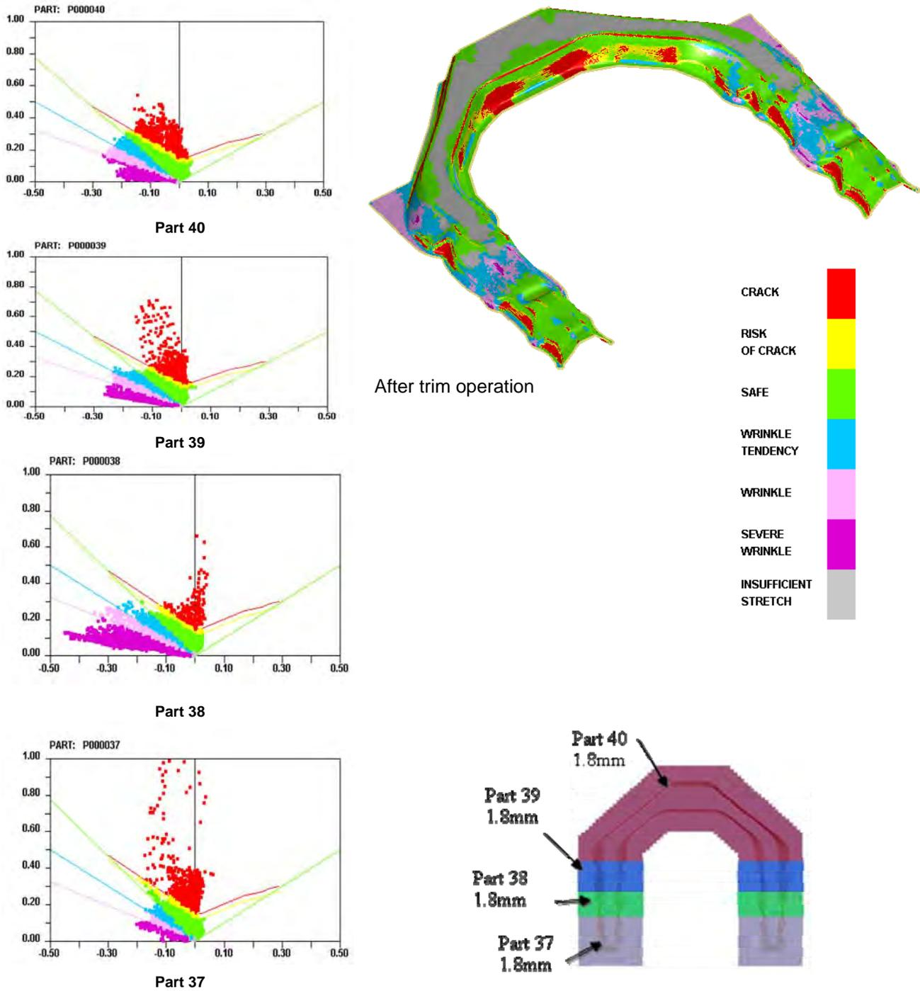
Figure2-6: Baseline FSV T5 Design Upper Rail Forming Results
