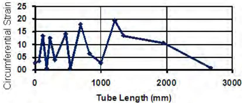
**Figure 12.31:** Final design hydroformed tube concept - circumferential strain
