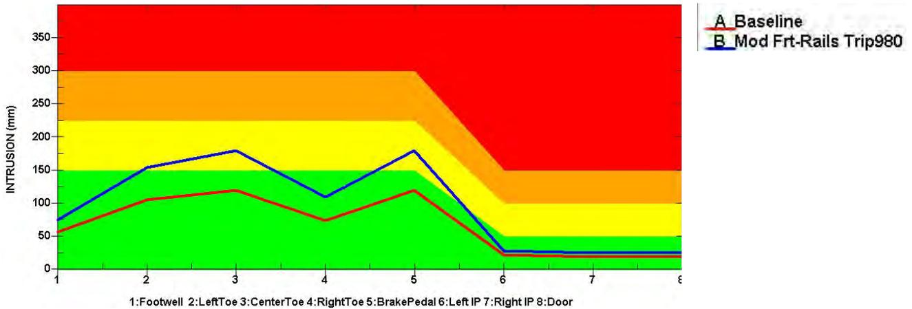
Figure 2-21: Modified Geometry IIHS ODB Performance Compared to Baseline
