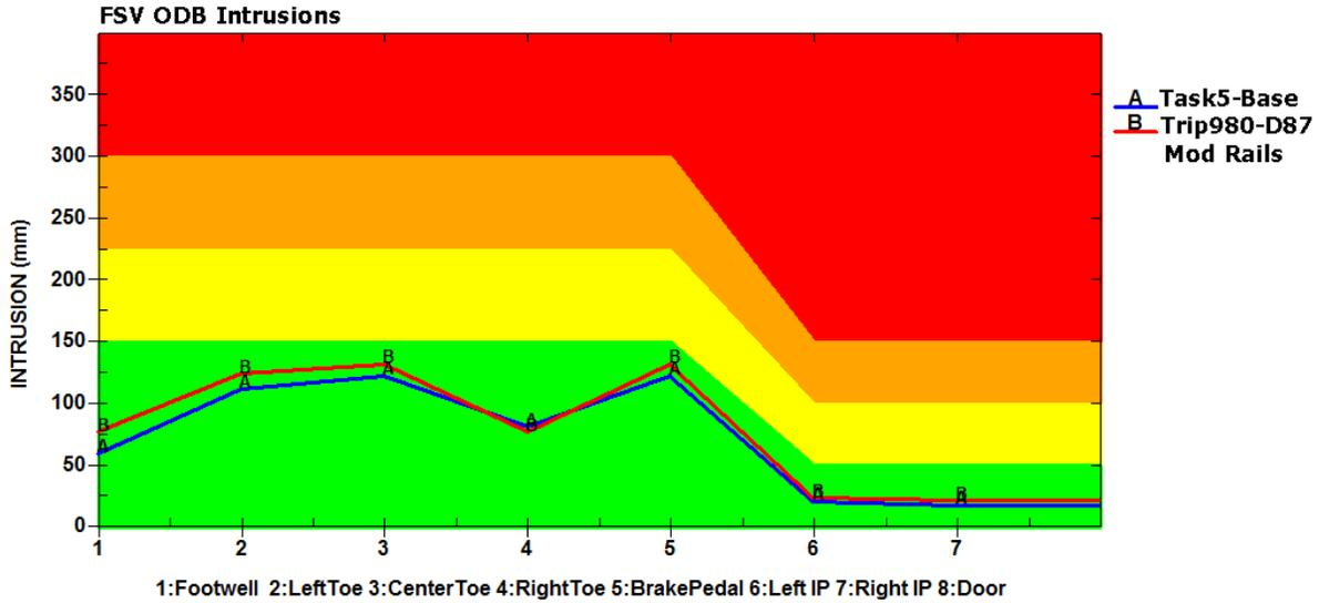
Figure 2-23: Results of Modified, Gauge Optimized Front Rails (red 'B' line) for IIHS ODB
