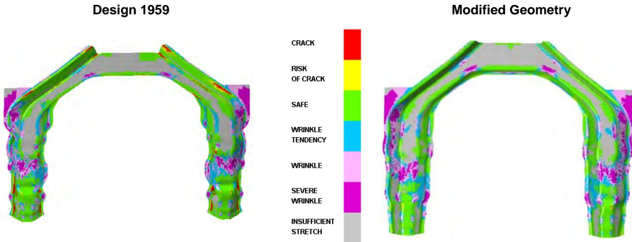
Figure 2-17: Upper Rail – 3B Forming Results on Modified Geometry
