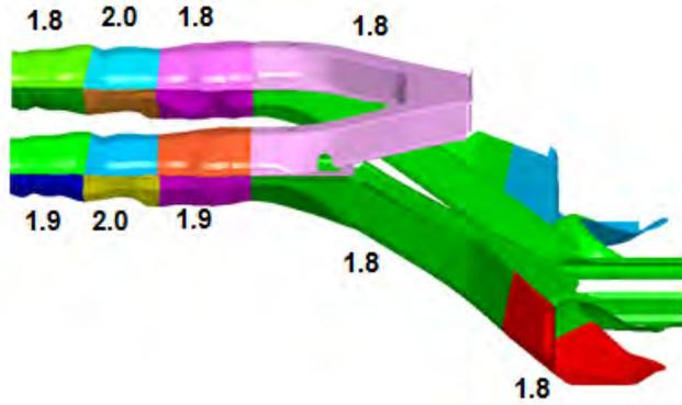
FSV T5 Front Rail Gauge Geometry
