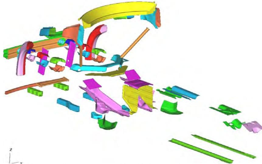
Figure 3-7: Components considered in front crash gauge optimization
