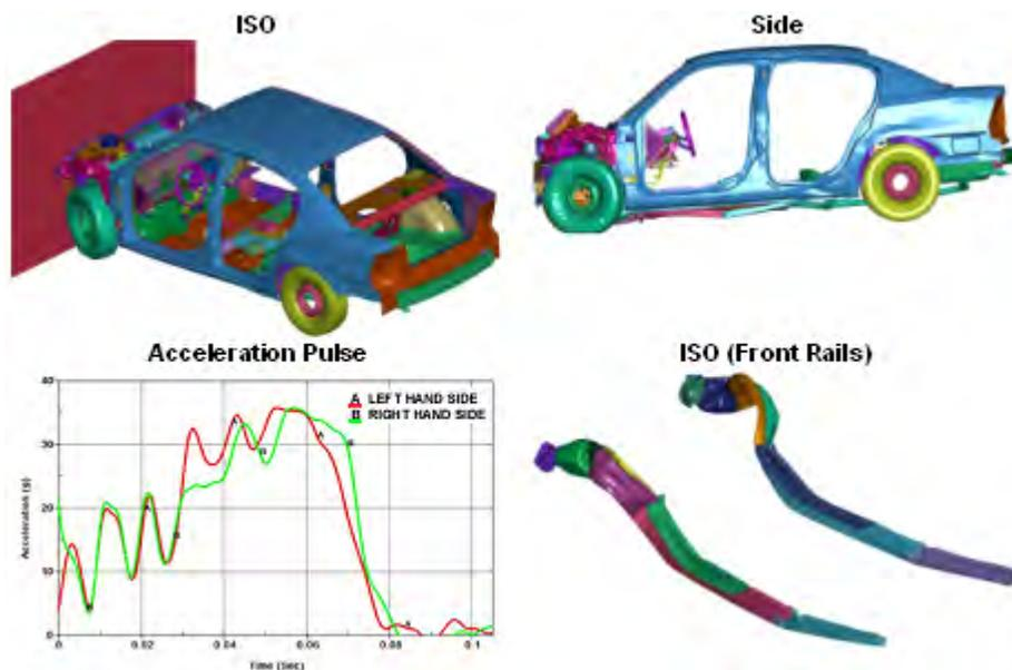
**Figure 12.6:** NCAP - deformed plots & acceleration
