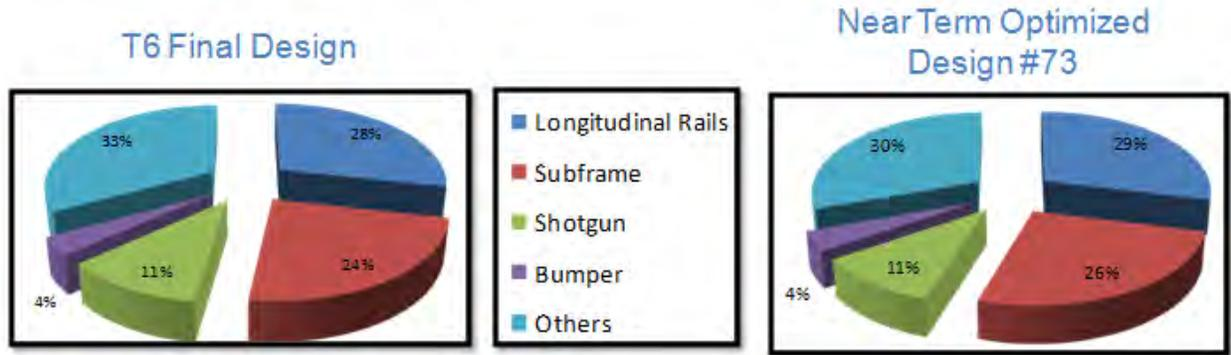
Figure 4-15: Energy Absorption Distribution (by percentage) of Key Load Management Components
